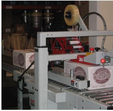
Before our line begins, we place our 6-pack carriers into case carriers. One person takes filled bottles from the line and places them into the prefilled case carriers. Once a case is filled with four 6-packs it is sent down another conveyor, through a cases sealer, to the final person on our line who indicates the style/brand and stacks the cases on a pallet.
