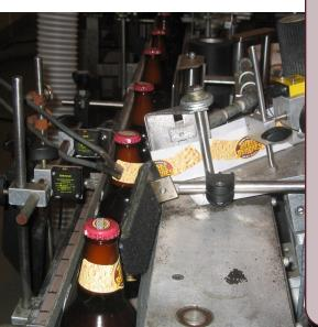
One person operates and adjusts the filler; adding crowns and ensuring it is functioning properly. This person also oversees the operation of the labeler, which includes changing rolls when necessary.
