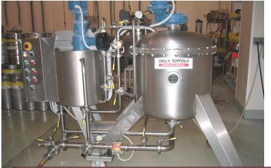
The beer is pumped from the fermenters through a diatomaceous earth particle filter. The filtration removes yeast and other particles that might limit the shelf life of the beer and to ensure beer clarity.
