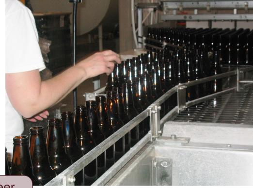
After filtration and carbonation, beer is then either filled into kegs or bottles.
